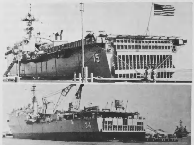
The USS PONCE (top), and the USS HERMITAGE (below), visited Aruba from Oct. 1-3. The USS Ponce is an Amphibious Transport Dock with a helicopter landing deck and hangar to house them. Underneath the landing deck is a floodable well for launching, receiving and transporting amphibious vehicles. The ship was built in 1971 and is on her first operational deployment to the Caribbean. Ariba ta USS PONCE, cu USS HERMITAGE (mas abao), cu a bishita Aruba Oct. 1-3.
